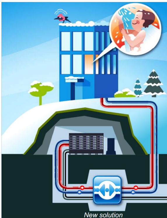
Picture 7. New cooling and waste heat solution in Academica Data Center.
